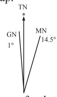
The compass needs to be adjusted to account for the magnetic declination (more in the compass section)
