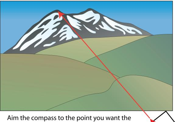
Aim the compass to the point you want the bearing, maintain it level so that the needle is free of movement, do not have any other metalic item close (car, pocket knife, other compass, watch, ski pole, etc)
